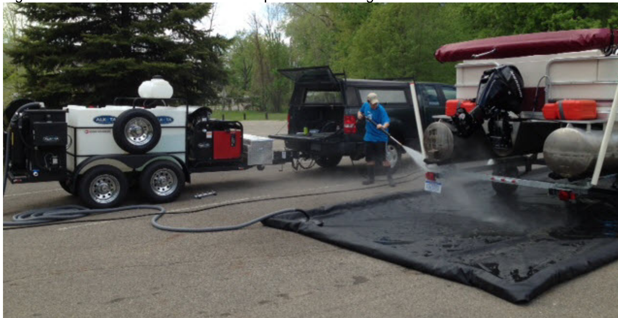
Figure 2: MDEQ's mobile boat wash in operation showing waste water containment
