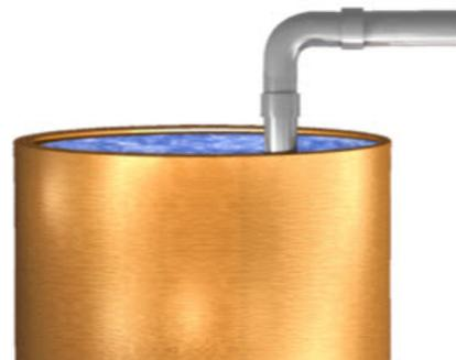
Typical Cross-Connection - Submerged Inlet
