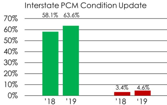
FHWA annually assesses the percent of Interstate pavement in poor condition to ensure compliance with a minimum condition level requirement that no more than five percent of the Interstate System be in poor condition. Per the Interstate Pavement Condition Measure data submitted to HPMS for the years 2018 and 2019, Michigan achieved the National Interstate Pavement Condition Goal, as no more than 5 percent of NHS pavements were in poor condition.
